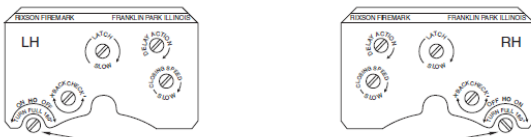
This Set Screw Is On Selector Hold-open Types Only
