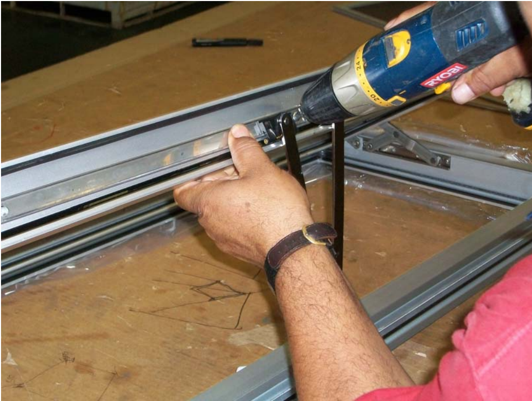
7. Attach tracks to vent
