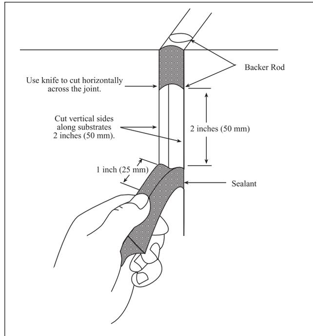
**NOTE:** When a sealant is used to weatherseal between two dissimilar substrates, it is recommended that the sealant adhesion to each side of the joint be individually tested. (See step e.)
