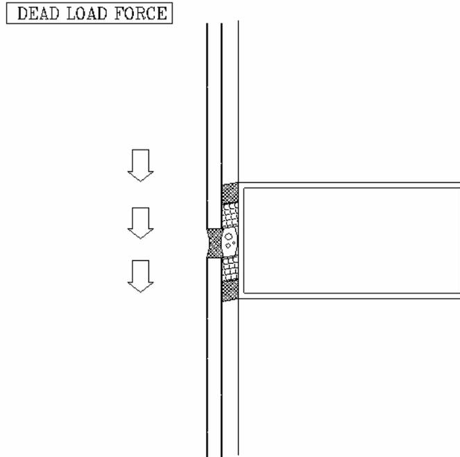
The deadload structural bite requirement is calculated as follows:
